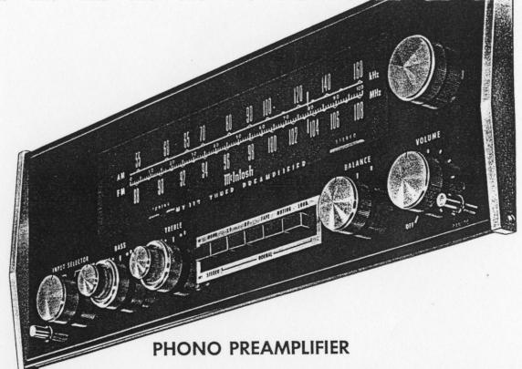
There are three transistors in each channel of the phono preamplifier. The output of the third transistor is connected by a negative feedback loop to the emitter of the input transistor. The feedback loop reduces noise and distortion. It also provides precision RIAA frequency compensation required for magnetic phonograph cartridges. Feedback remains in effect even at 20 Hz, where gain is highest. The negative feedback also provides a low output impedance for the tape output.
